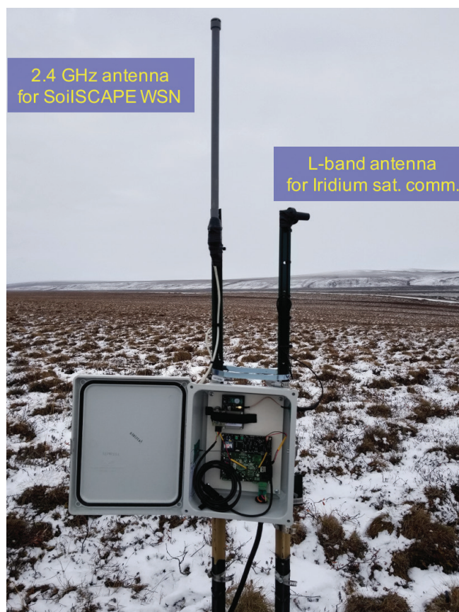
A SoilSCAPE base station (coordinator) at an Alaska site. The coordinator receives data from the SoilSCAPE probes (the wireless sensor network, or WSN) and sends it to the lab via satellite. The coordinator also receives commands from the lab and relays them to the SoilSCAPE sensors using the same communication path in reverse.
