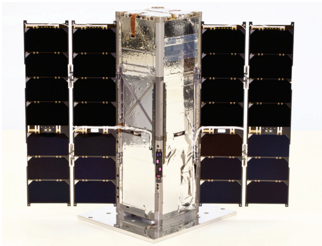
The RAVAN CubeSat successfully demonstrated new technologies to measure Earth's radiation imbalance and predict future climate change (Image credit: JHU APL/Blue Canyon Technologies)
