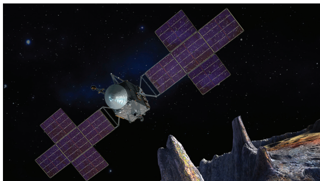
NASA's Psyche mission carries a gamma-ray detector to measure the elemental composition of the asteroid 16 Psyche (Image credit: NASA/Arizona State University).
