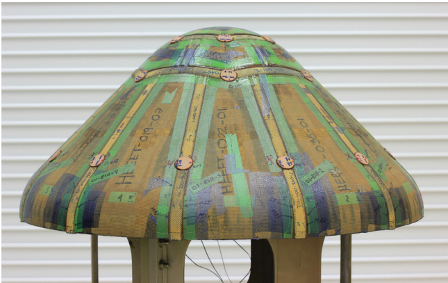
HEEET Engineering Test Unit (ETU) prior to final surface machining
