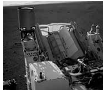
RPS have enabled numerous NASA missions over the last five decades, including the Mars Science Laboratory launched in November 2011. The Curiosity rover took this image showing its Multi-Mission Thermoelectric Generator (MMRTG) on the surface of Mars on Aug. 7, 2012.
