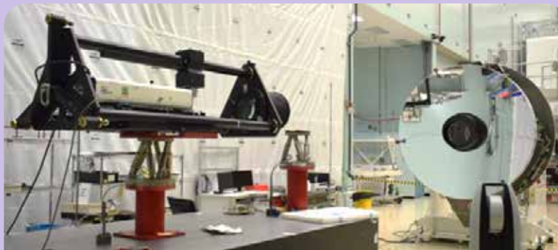
Primary Mirror horizontal optical test
